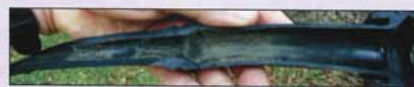
Figure 4. Worn liners will greatly increase the spread of Staph aureus between cows. This liner had carried over 8,000 milkings.
