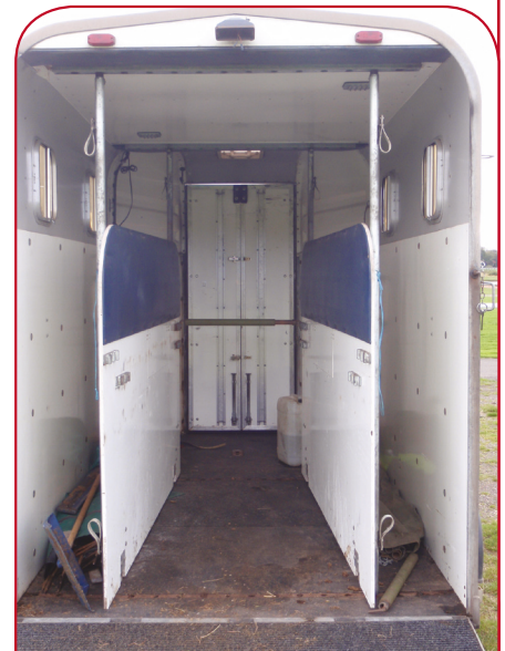
A HORSE AMBULANCE PROVIDES A LOW RAMP AND SUPPORTING PARTITIONS FOR EASE OF LOADING AND TRANSPORT
